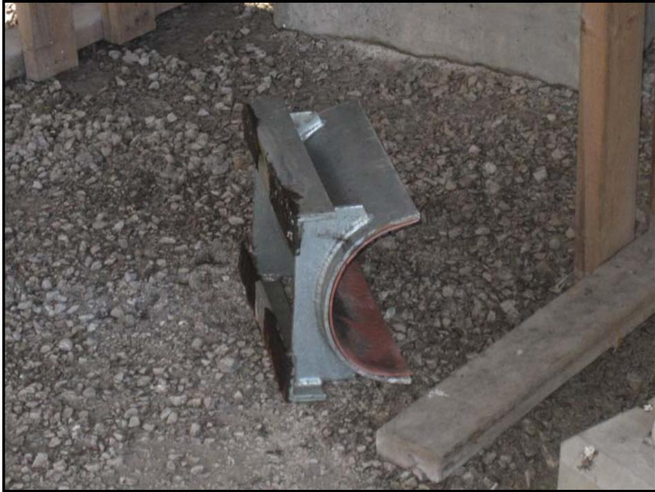
Excessive pipe movement allowed support to fall from bridge. Cause of the black areas on slides is unknown.
